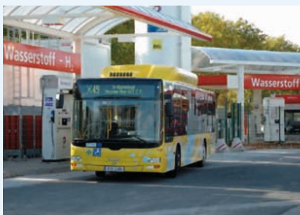
Hydrogen refilling station in Berlin which uses LPG as its feedstock. The facility was created within the framework of the European Commission's 6 th framework programme on research.
